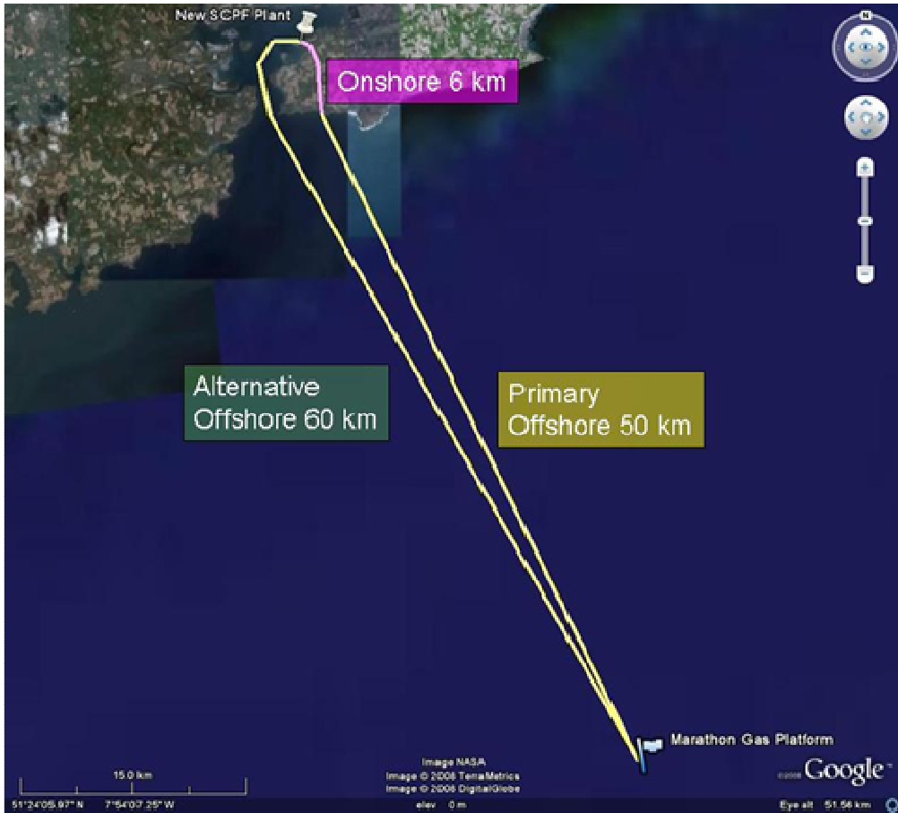
Figure 16 – Proposed pipeline route from the 900 MW e power station at Cork to Kinsale Head gas field
