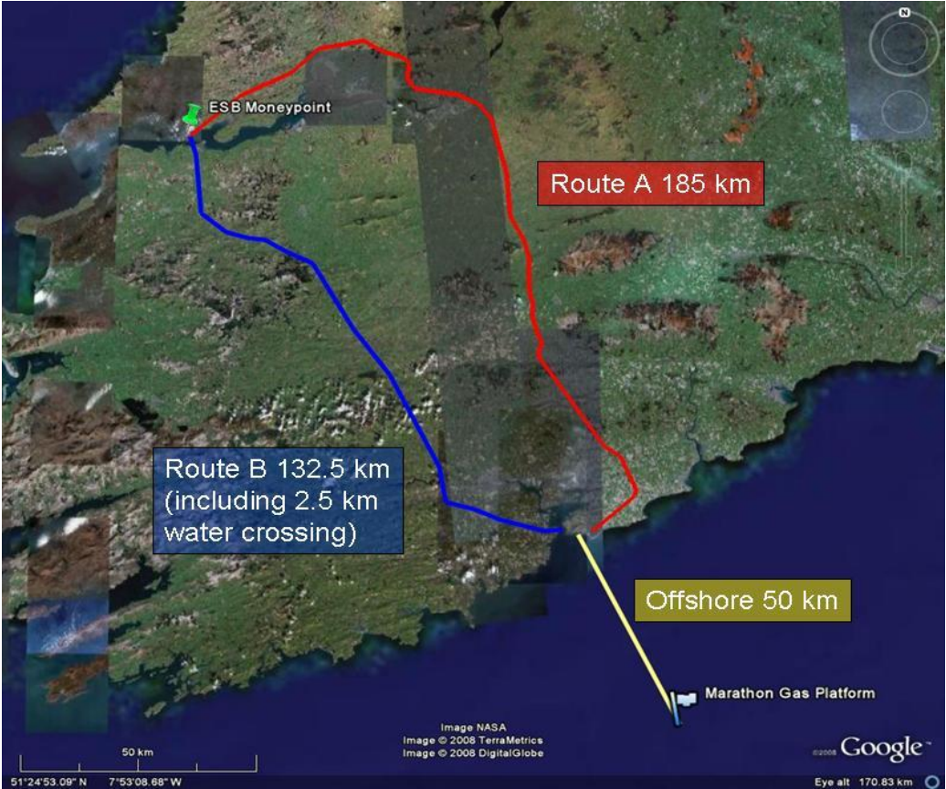
Figure 5 – Proposed pipeline route (Route A) from Moneypoint Power station to Kinsale Head depleted gas field
