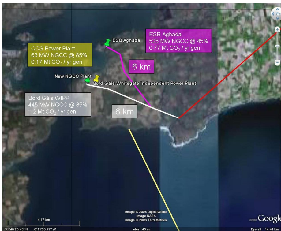
Figure 15 – Proposed pipeline route from the retrofitted power stations at Cork to the main Moneypoint CCS pipeline
