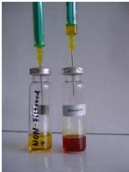
Fig. 3: Quick test for acid value, showing the indicator colours before, during and after the titration reaction.
