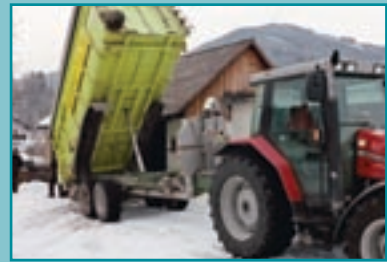
Purpose built wood chip trailer that blows wood chips into a fuel bunker.
