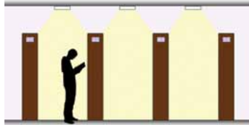
Fig.4b Light distribution for shelving
