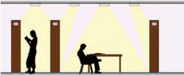
Fig.4a Light distribution for shelving and task areas
